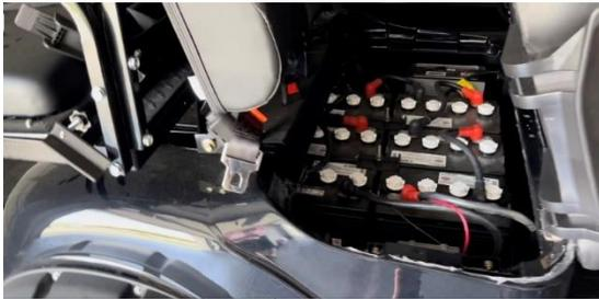
the same energy storage need. Note an example in the photo to the left of a golf cart with its typical array of 6 batteries weighing in at 470 pounds.
